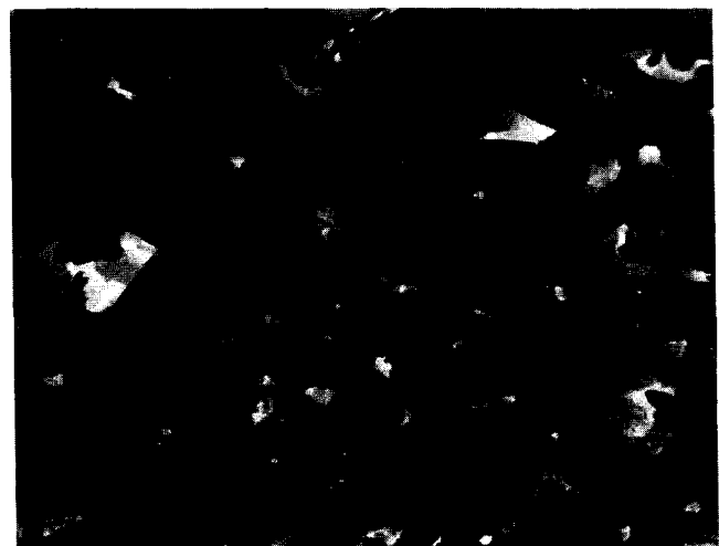
Fig. 4. Positive paste 3 before formation.
