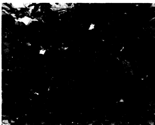
Fig. 8. Positive paste 3 after formation.
